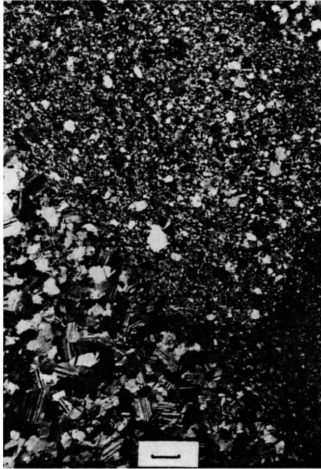
Fig. 1. Variation in microstructure across a shear zone boundary in the borehole shear zone. The fine grained plagioclase marks the mylonite in the shear zone. Scale bar = 1 mm.
